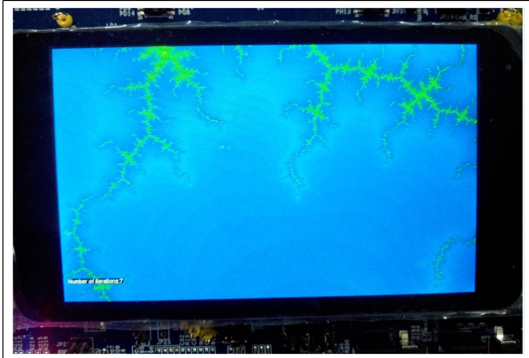
Figure 7. Picture of Mandelbrot-set using Single precision FPU with zoom in 32 times
