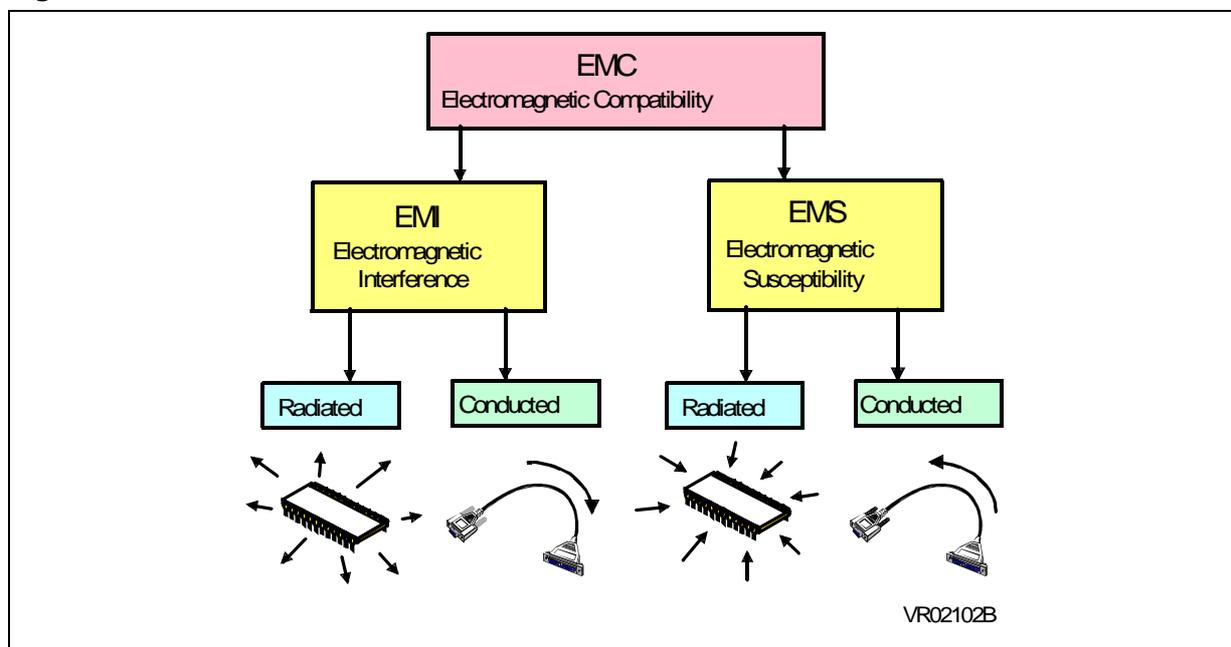
**Electromagnetic interference (EMI)** tests involve measuring the frequency and amplitude of undesirable signals emitted by the tested equipment. Signal radiated into free space are called **radiated emissions**, whereas signals travelling along power cords or other interconnecting cables are called **conducted emissions**.
