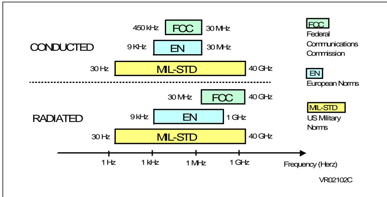
**EMC regulations** cover the entire spectrum of electrical products, from computing equipment to microwave ovens to aircraft. As shown, the frequency ranges of interest for EMC testing extend from **30 Hz to 40 GHz** (9 orders of magnitude), depending on the agency and the type of measurement. The frequency range over which regulations exist varies, depending on the device and its intended use.
