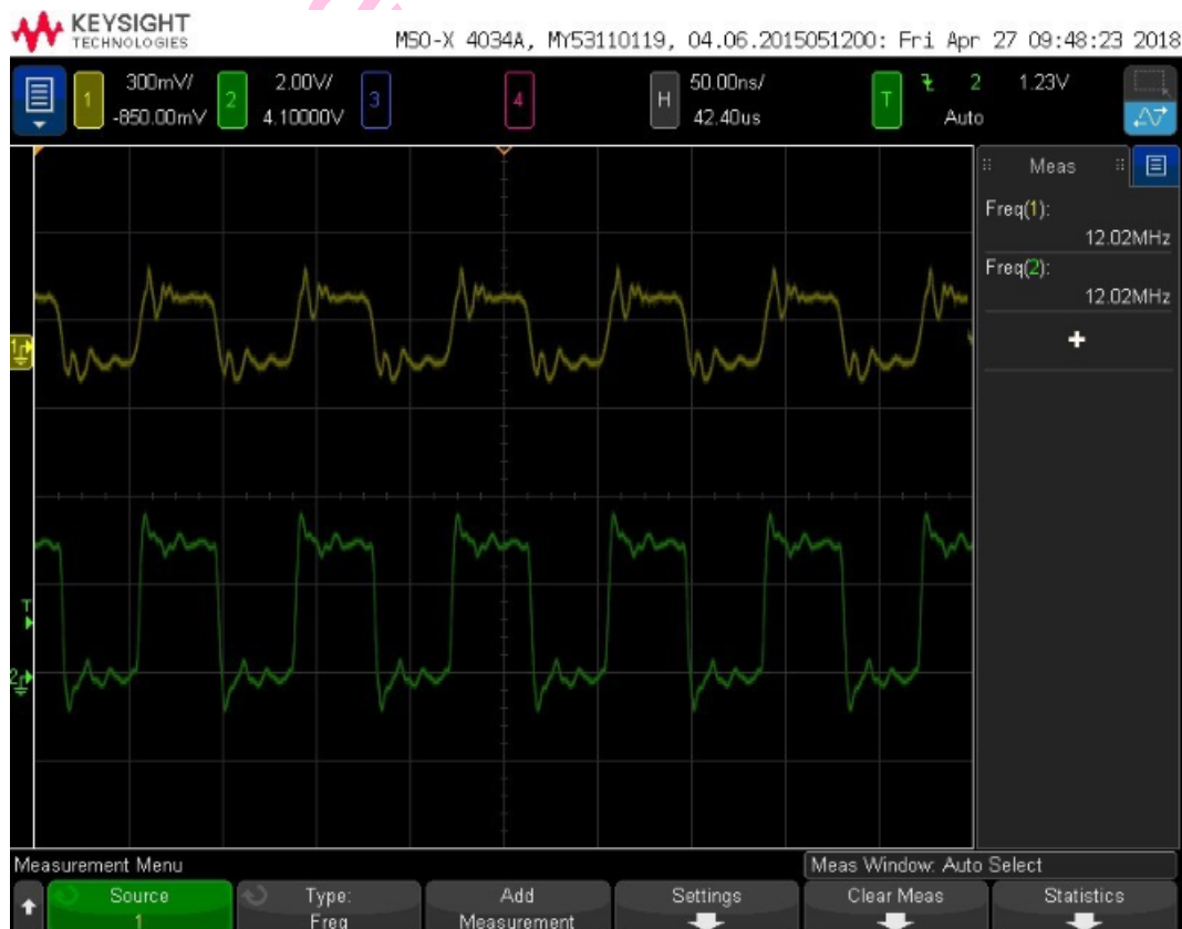
Figure 18. Receiver input and output waveforms
