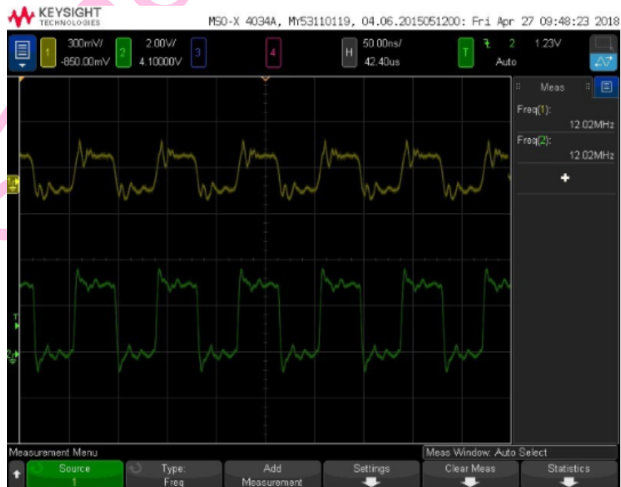
Figure 20. Comparator input and output waveforms
