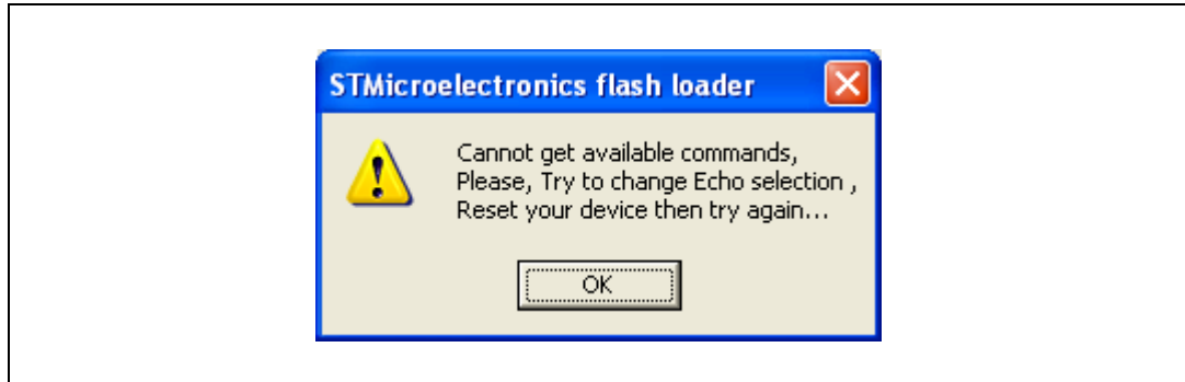
Figure 3. Dialog message if experiencing problems when trying to connect to the device with the Flash loader demonstrator
