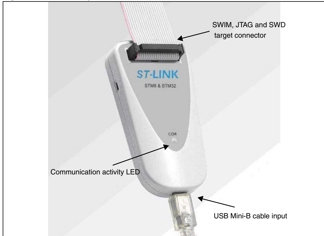
Figure 3. ST-LINK layout
