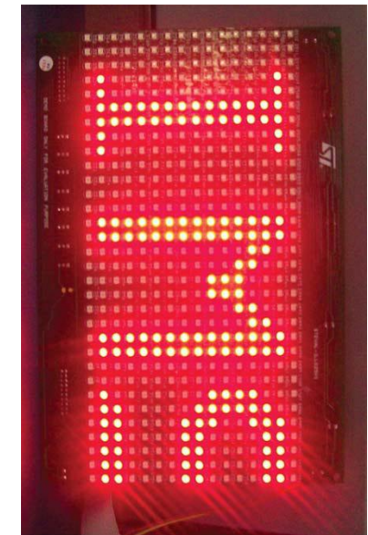
STEVAL-ILL025V1 shows capability of STP16DP05 in driving LED matrix display panel
