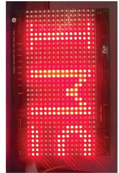
STEVAL-ILL025V1 shows capability of STP16DP05 in driving matrix LED display panel
