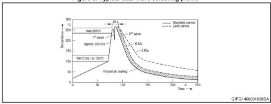
Figure 6: Typical dual-wave soldering profile
