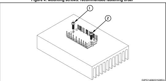
Figure 4: Mounting screws: recommended fastening order
