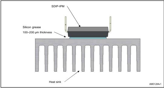
Figure 1: Recommended silicon grease thickness
