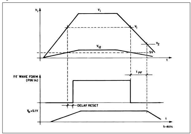
The energy which the filter capacitor C supplies to the operating device while it discharges is :  $E = 1/2 \text{ C } (V_1^2 - V_2^2)$
