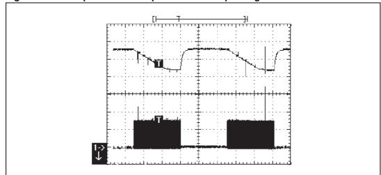
Figure 4. Example: L6385E output and bootstrap voltage
