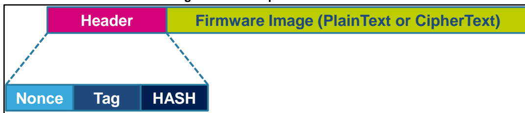
Figure 14: FOTA packet structure
