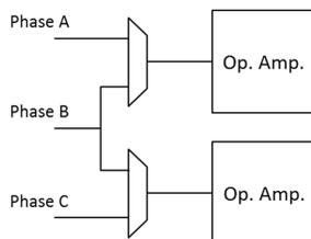
It's easy to see that the perfect choice, the one that minimizes - down to three - the pincount, is to select PA1, PA7, PB0: signals coming from the three shunts U-V-W, connected to these pins, are served by three different comparators and can be amplified simultaneously by two comparators in any combination (UV, VW, UW).
