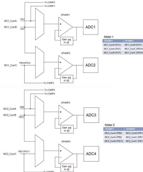
Table 2 shows a possible solution for dual motor control in triple sampling mode. The inputs of the three op amps must be switched on-the-fly between the three pairs of inputs.
