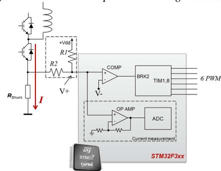
In Figure 4 is shown the over-current protection network that can be implemented using the internal resources of the STM32F30x. Phase current measurement and overcurrent protection share the same microcontroller pin.
