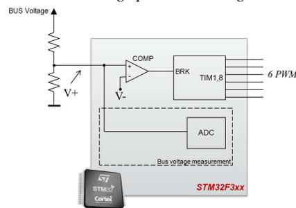
In Figure 5 is shown the over-voltage protection network that
