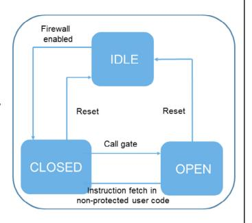
The Firewall is based on 3 states to ensure a dynamic protection of the secure segments. The Idle state is the default state when the Firewall is not enabled. In this state, the AHB memory bus is not monitored. When enabled, the Firewall enters Closed state and all access to the protected segments is prohibited.
