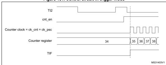
Figure 131. Control circuit in trigger mode
