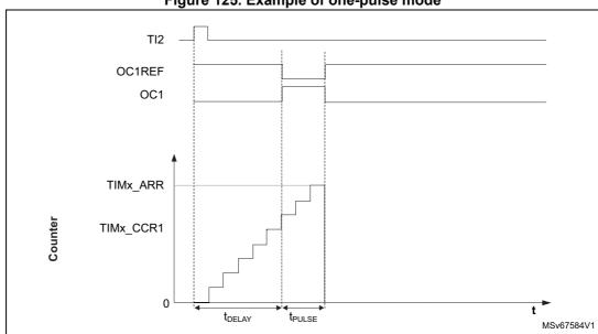
Figure 125. Example of one-pulse mode
