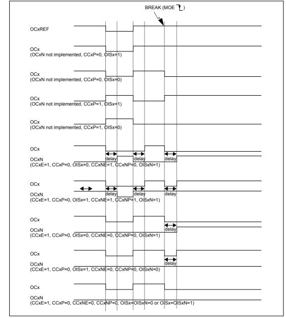
Figure 82. Output behavior in response to a break
