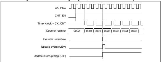
Figure 56. Counter timing diagram, internal clock divided by 4
