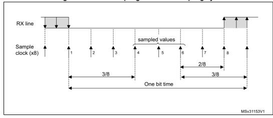
Figure 236. Data sampling when oversampling by 8
