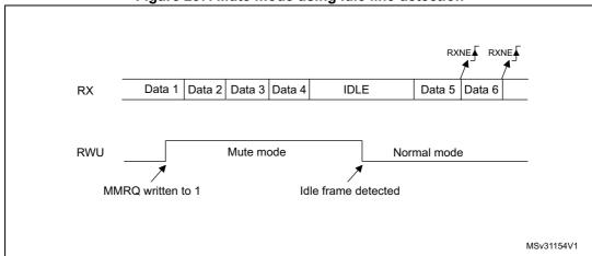
Figure 237. Mute mode using Idle line detection
