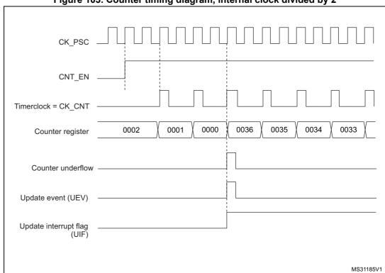
Figure 103. Counter timing diagram, internal clock divided by 2
