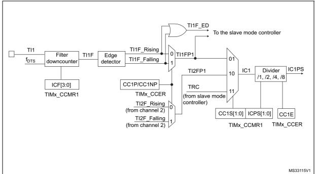
Figure 71. Capture/compare channel (example: channel 1 input stage)
