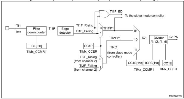
Figure 178. Capture/compare channel (example: channel 1 input stage)
