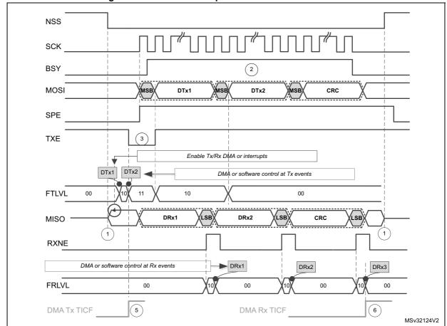
Figure 261. Master full-duplex communication with CRC
