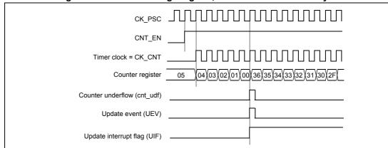
Figure 54. Counter timing diagram, internal clock divided by 1
