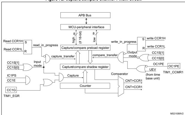
Figure 72. Capture/compare channel 1 main circuit
