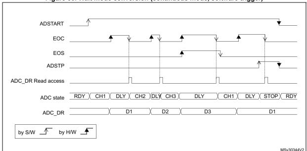
Figure 36. Wait mode conversion (continuous mode, software trigger)
