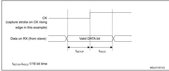
Figure 242. RX data setup/hold time
