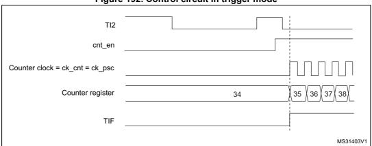
Figure 192. Control circuit in trigger mode
