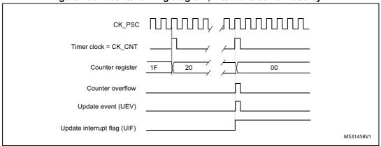
Figure 156. Counter timing diagram, update event when ARPE=0 (TIMx\_ARR not preloaded)
