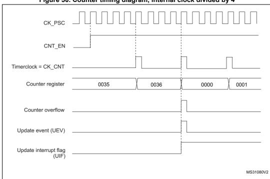
Figure 50. Counter timing diagram, internal clock divided by 4
