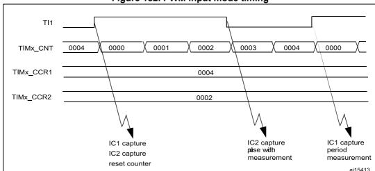
Figure 182. PWM input mode timing
