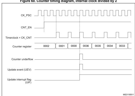
Figure 60. Counter timing diagram, internal clock divided by 2
