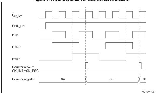
Figure 117. Control circuit in external clock mode 2
