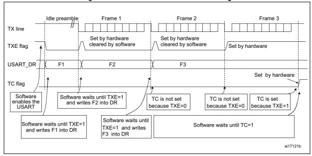
Figure 233. TC/TXE behavior when transmitting
