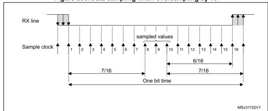
Figure 235. Data sampling when oversampling by 16
