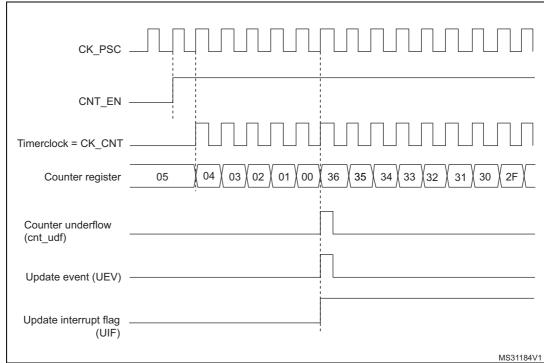
Figure 102. Counter timing diagram, internal clock divided by 1
