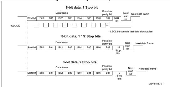
Figure 232. Configurable stop bits
