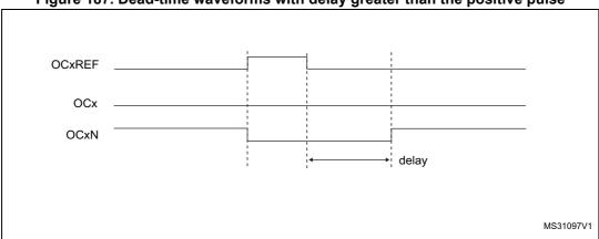
The dead-time delay is the same for each of the channels and is programmable with the DTG bits in the TIMx\_BDTR register. Refer to Section 17.5.16: TIM15 break and dead-time register (TIM15\_BDTR) on page 446 for delay calculation.
