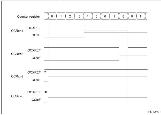
Figure 77. Edge-aligned PWM waveforms (ARR=8)
