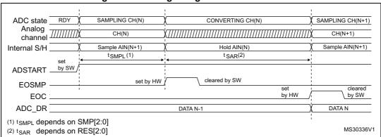
Figure 28. ADC conversion timings
