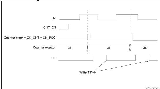
Figure 177. Control circuit in external clock mode 1
