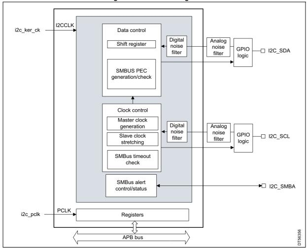
Figure 199. I2C block diagram
