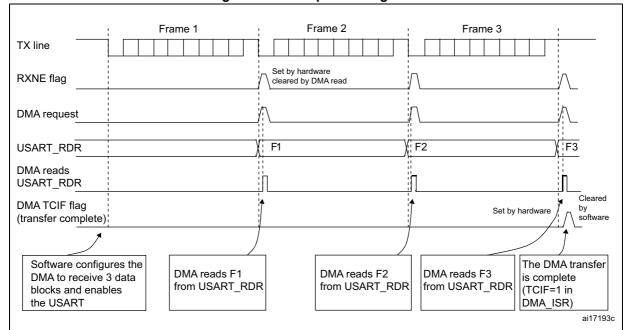
Figure 244. Reception using DMA
