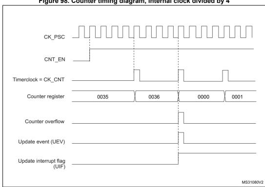
Figure 98. Counter timing diagram, internal clock divided by 4
