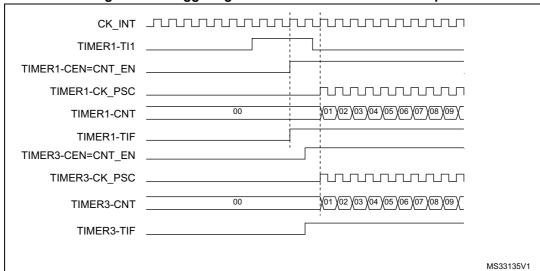
Figure 138. Triggering timer 1 and 3 with timer 1 TI1 input
