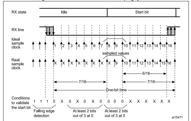
Figure 234. Start bit detection when oversampling by 16 or 8
