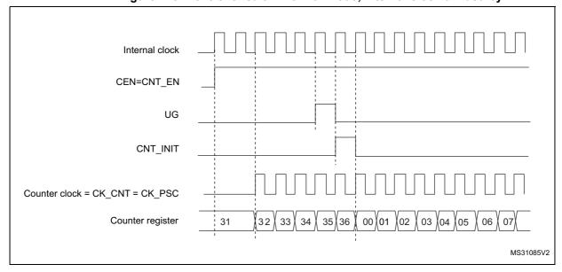
Figure 175. Control circuit in normal mode, internal clock divided by 1
