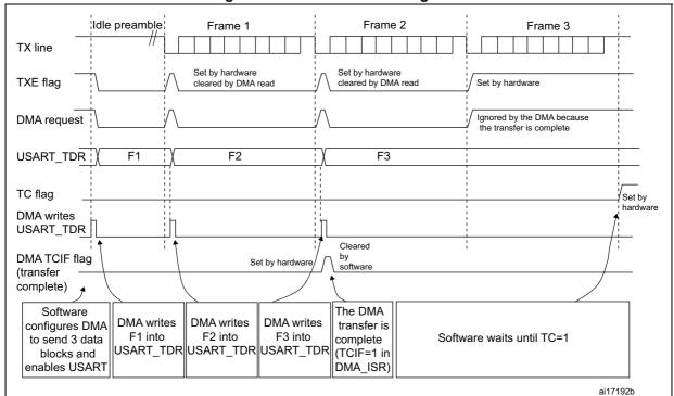
Figure 243. Transmission using DMA
