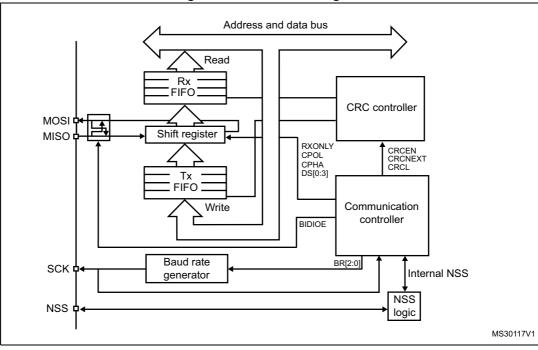
Figure 249. SPI block diagram
