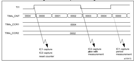
Figure 121. PWM input mode timing
