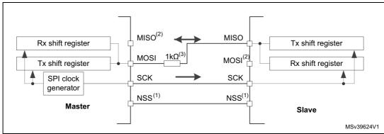
Figure 251. Half-duplex single master/ single slave application
