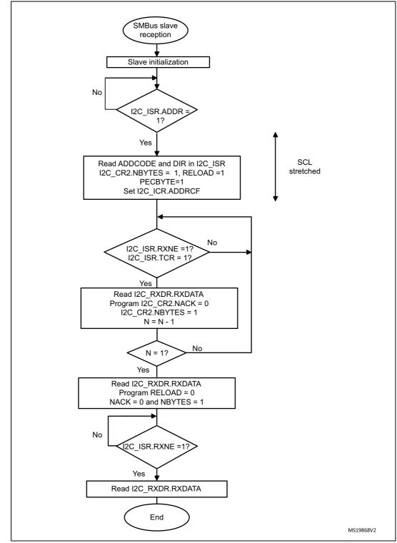
Figure 226. Transfer sequence flow for SMBus slave receiver N bytes + PEC
