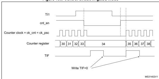
Figure 130. Control circuit in gated mode
