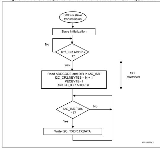
Figure 224. Transfer sequence flow for SMBus slave transmitter N bytes + PEC
