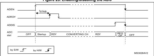
Figure 25. Enabling/disabling the ADC
