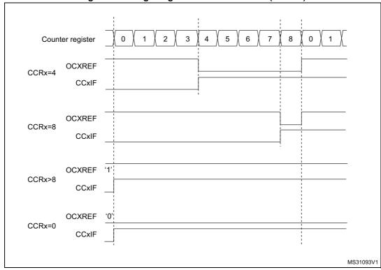
Figure 163. Edge-aligned PWM waveforms (ARR=8)
