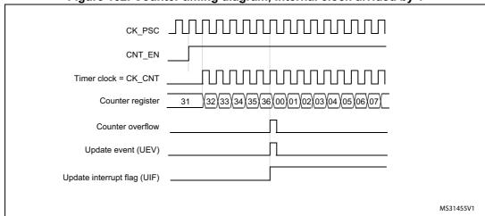
Figure 152. Counter timing diagram, internal clock divided by 1
