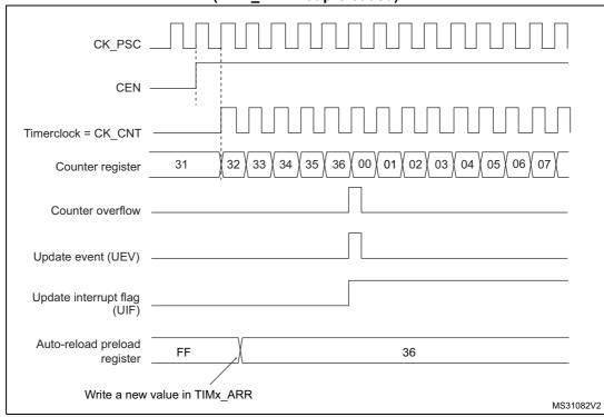
Figure 100. Counter timing diagram, Update event when ARPE=0 (TIMx\_ARR not preloaded)
