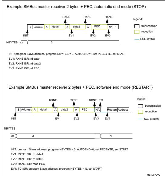
Figure 229. Bus transfer diagrams for SMBus master receiver
