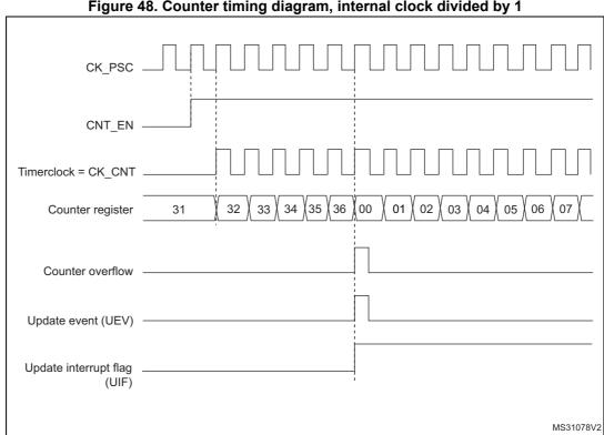
Figure 48. Counter timing diagram, internal clock divided by 1
