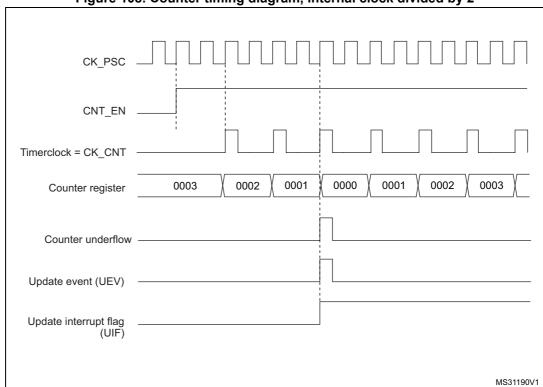
Figure 108. Counter timing diagram, internal clock divided by 2
