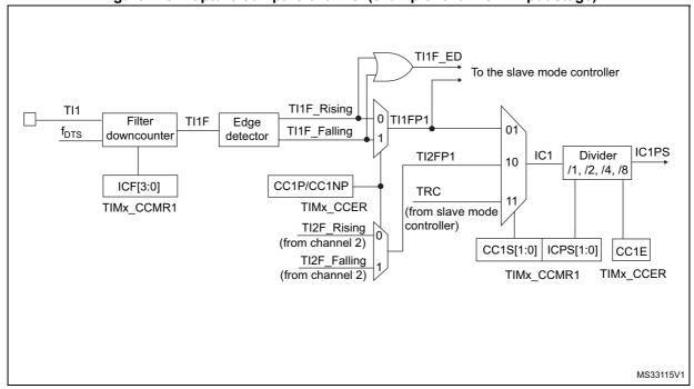
Figure 118. Capture/compare channel (example: channel 1 input stage)
