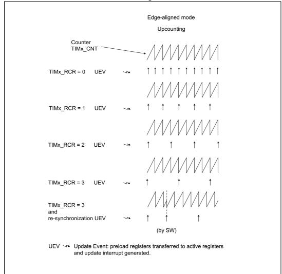
Figure 174. Update rate examples depending on mode and TIMx\_RCR register settings
