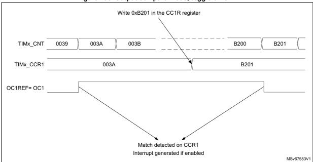
Figure 183. Output compare mode, toggle on OC1
