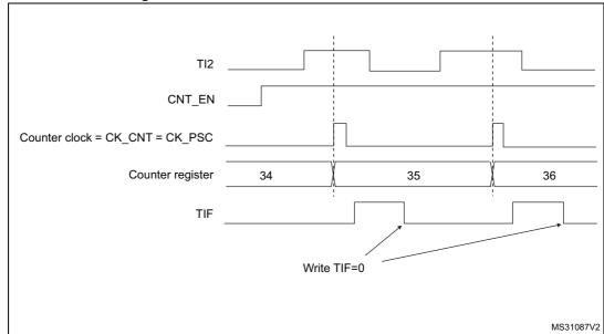
Figure 115. Control circuit in external clock mode 1
