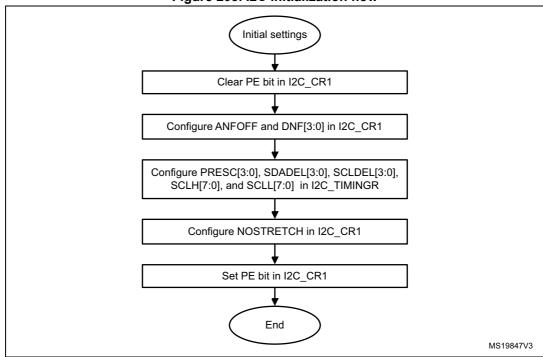
Figure 203. I2C initialization flow
