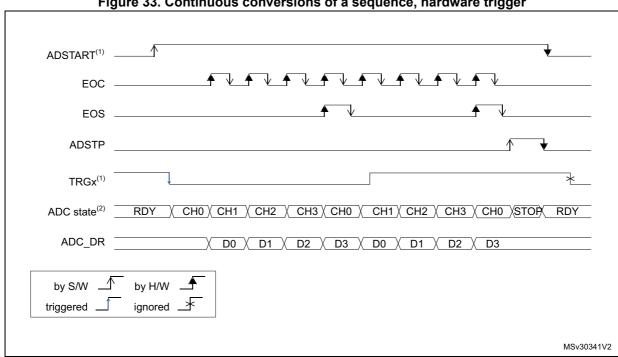
Figure 33. Continuous conversions of a sequence, hardware trigger
