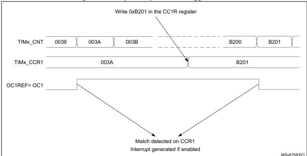
Figure 122. Output compare mode, toggle on OC1
