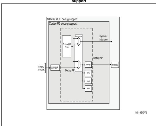
1. The debug features embedded in the Arm® Cortex®-M0 core are a subset of the Arm CoreSight Design Kit.
