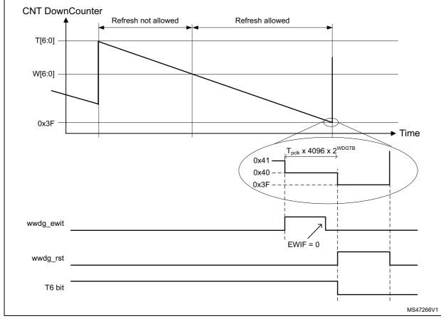
Figure 196. Window watchdog timing diagram
