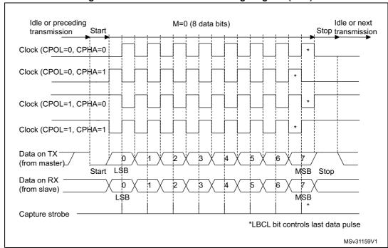
Figure 240. USART data clock timing diagram (M=0)
