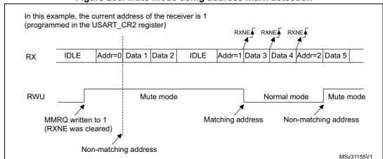
Figure 238. Mute mode using address mark detection
