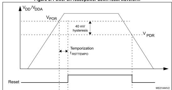
Figure 8. Power on reset/power down reset waveform
