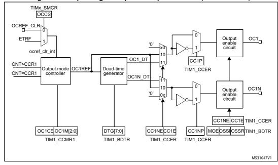
Figure 73. Output stage of capture/compare channel (channel 1 to 3)
