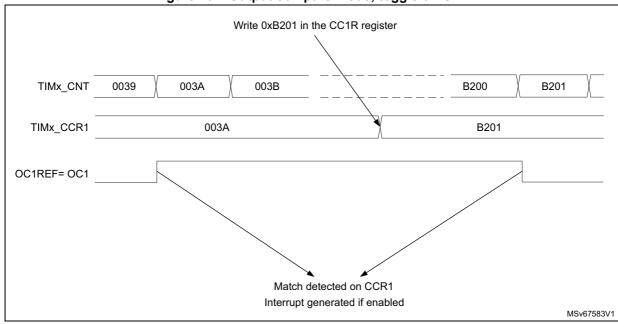
Figure 162. Output compare mode, toggle on OC1
