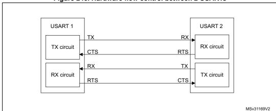
Figure 245. Hardware flow control between 2 USARTs
