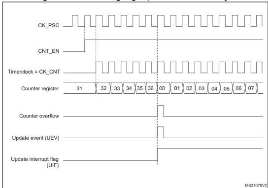
Figure 168. Counter timing diagram, internal clock divided by 1
