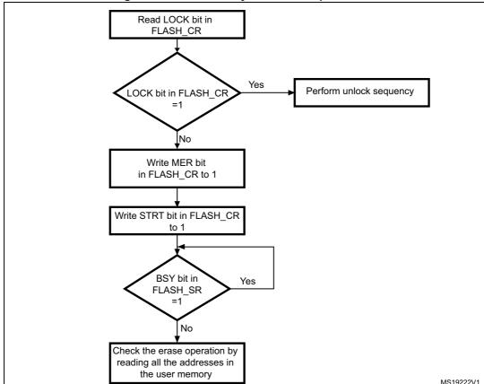
Figure 5. Flash memory mass erase procedure
