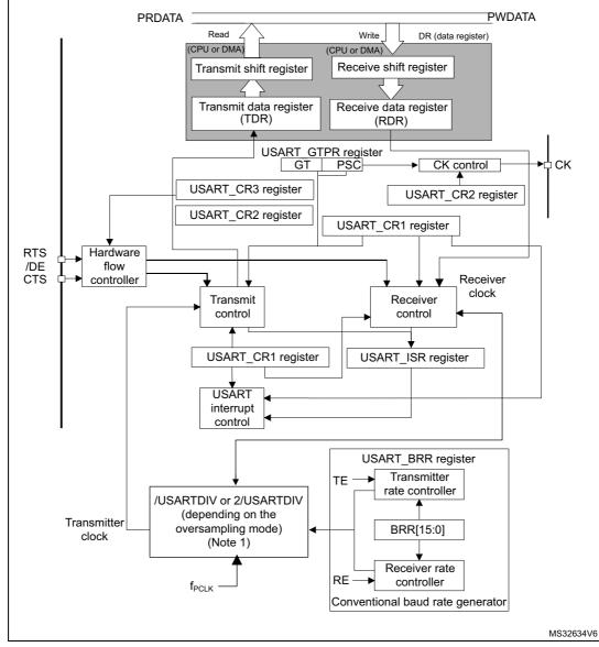
Figure 230. USART block diagram
