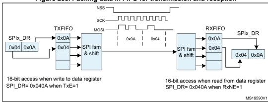
Figure 258. Packing data in FIFO for transmission and reception
