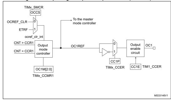
Figure 120. Output stage of capture/compare channel (channel 1)
