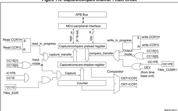
Figure 119. Capture/compare channel 1 main circuit
