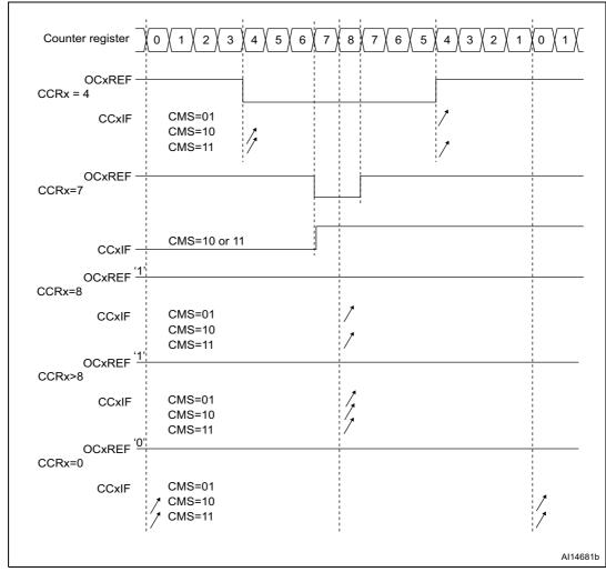
Figure 124. Center-aligned PWM waveforms (ARR=8)
