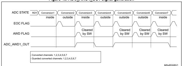
Figure 40. ADC\_AWD1\_OUT signal generation
