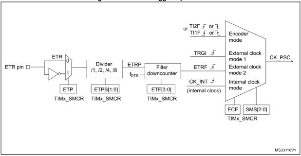
Figure 69. External trigger input block
