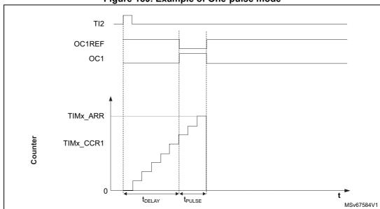
Figure 189. Example of One-pulse mode
