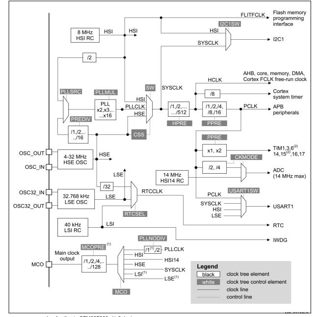
Figure 10. Clock tree (STM32F030x4, STM32F030x6 and STM32F030x8 devices)
