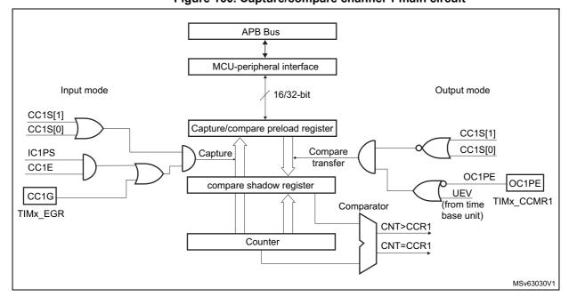
Figure 160. Capture/compare channel 1 main circuit
