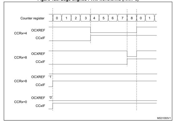
Figure 123. Edge-aligned PWM waveforms (ARR=8)
