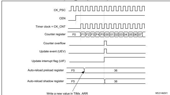
Figure 157. Counter timing diagram, update event when ARPE=1 (TIMx\_ARR preloaded)
