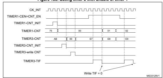
Figure 135. Gating timer 3 with Enable of timer 1
