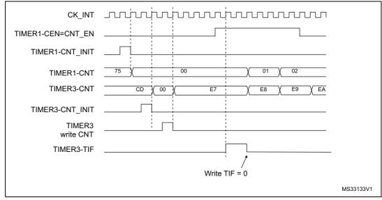
Figure 137. Triggering timer 3 with Enable of timer 1
