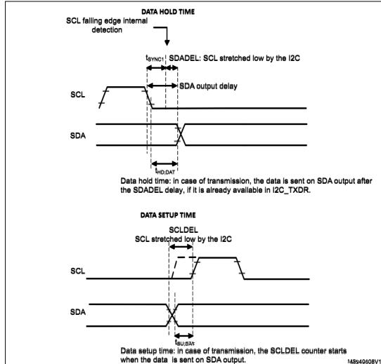
Figure 202. Setup and hold timings
