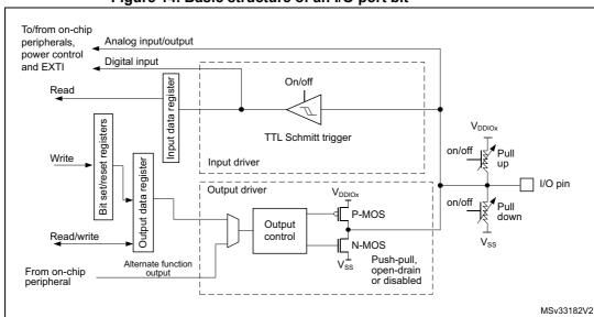
Figure 14. Basic structure of an I/O port bit
