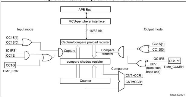
Figure 179. Capture/compare channel 1 main circuit
