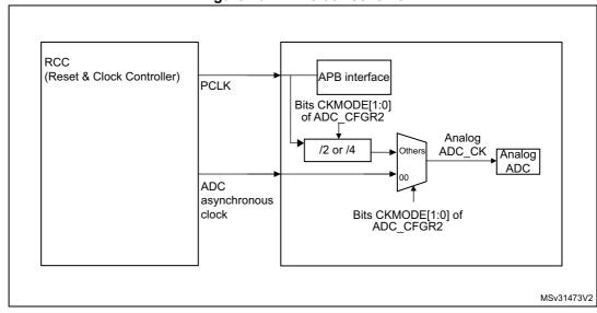
Figure 26. ADC clock scheme
