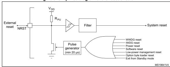
Figure 9. Simplified diagram of the reset circuit
