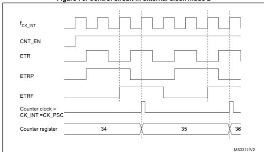
Figure 70. Control circuit in external clock mode 2
