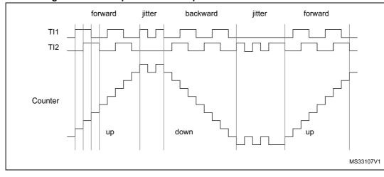
Figure 127. Example of counter operation in encoder interface mode
