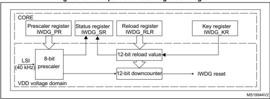
Figure 194. Independent watchdog block diagram
