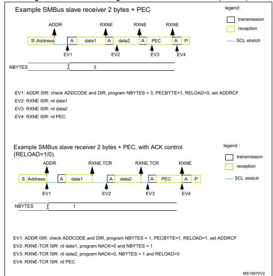
Figure 227. Bus transfer diagrams for SMBus slave receiver (SBC = 1)
