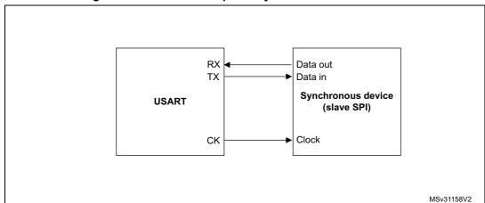
Figure 239. USART example of synchronous transmission
