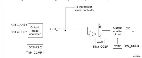
Figure 161. Output stage of capture/compare channel (channel 1)
