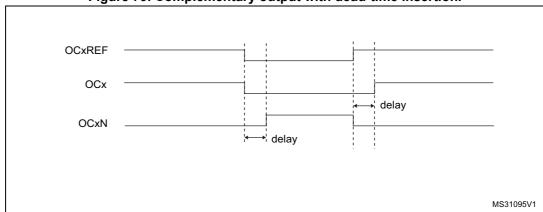
Figure 79. Complementary output with dead-time insertion.
