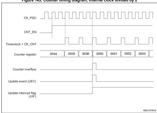
Figure 143. Counter timing diagram, internal clock divided by 2
