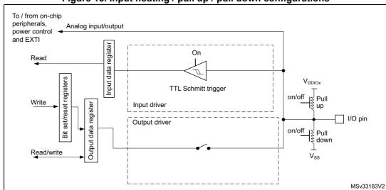
Figure 15. Input floating / pull up / pull down configurations
