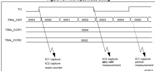
Figure 75. PWM input mode timing
