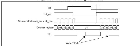
Figure 90. Control circuit in gated mode
