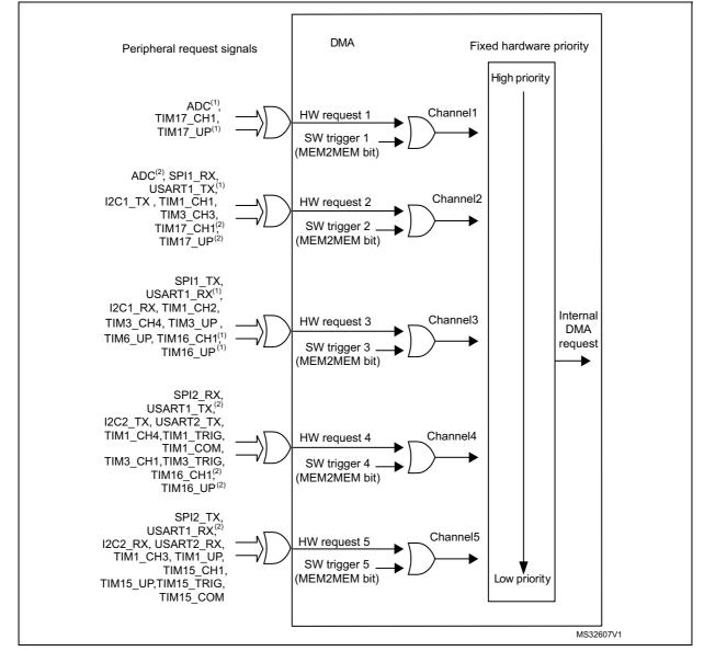
Figure 19. DMA request mapping
