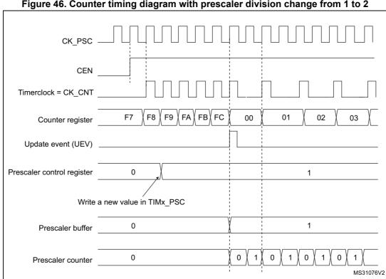
Figure 46. Counter timing diagram with prescaler division change from 1 to 2
