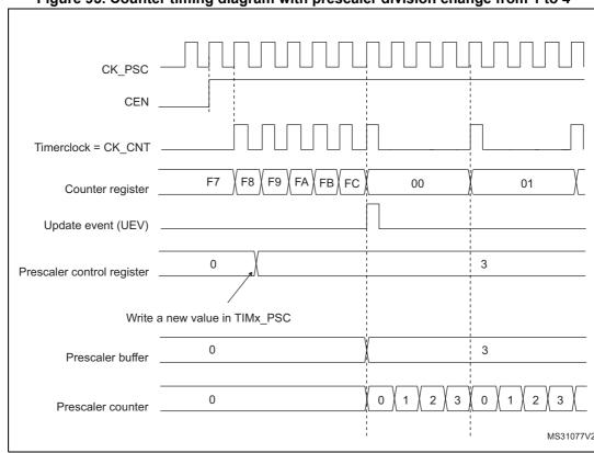
Figure 95. Counter timing diagram with prescaler division change from 1 to 4
