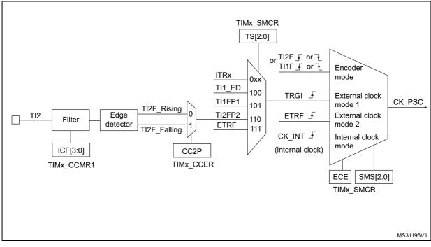
Figure 114. Tl2 external clock connection example
