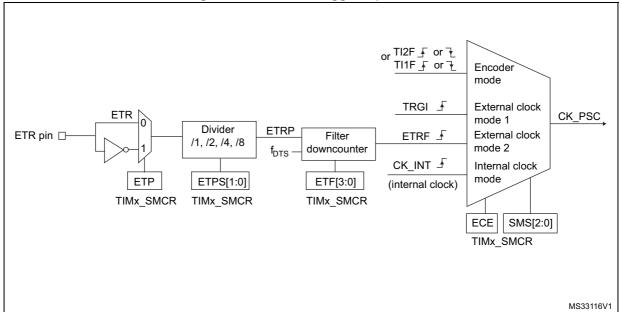
Figure 116. External trigger input block
