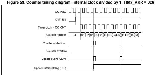
Here, center-aligned mode 1 is used (for more details refer to Section 13.4: TIM1 registers on page 272).
