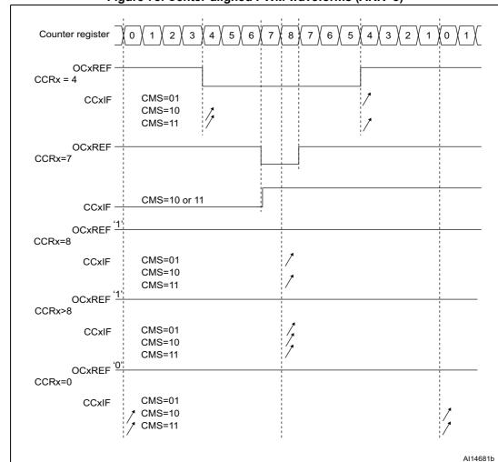
Figure 78. Center-aligned PWM waveforms (ARR=8)
