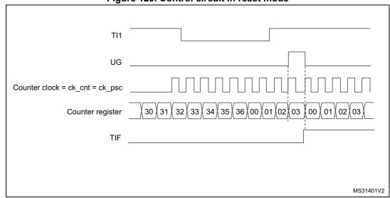
Figure 129. Control circuit in reset mode
