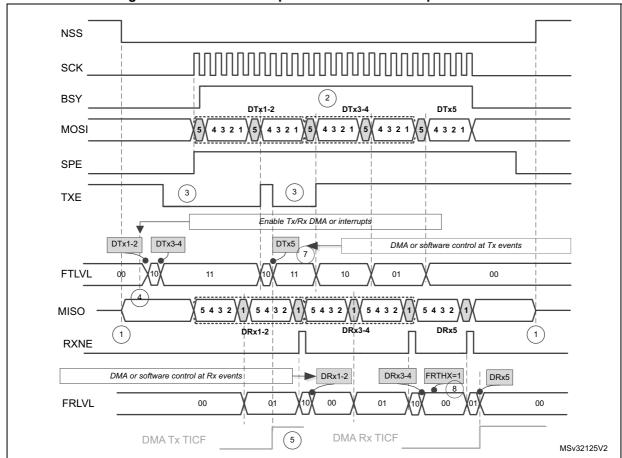
Figure 262. Master full-duplex communication in packed mode
