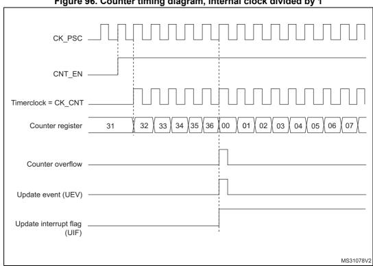
Figure 96. Counter timing diagram, internal clock divided by 1
