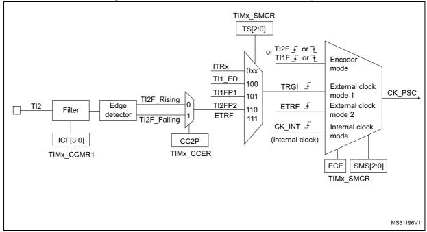
Figure 176. TI2 external clock connection example
