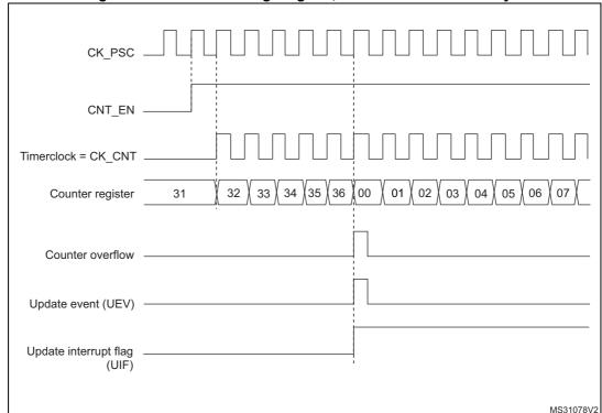
Figure 142. Counter timing diagram, internal clock divided by 1
