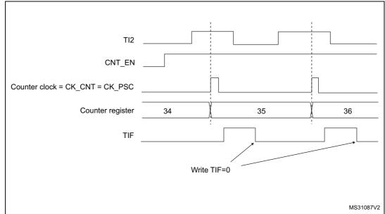
Figure 68. Control circuit in external clock mode 1
