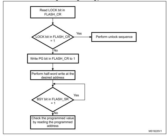
Figure 3. Programming procedure
