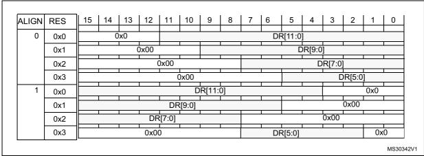
Figure 34. Data alignment and resolution
