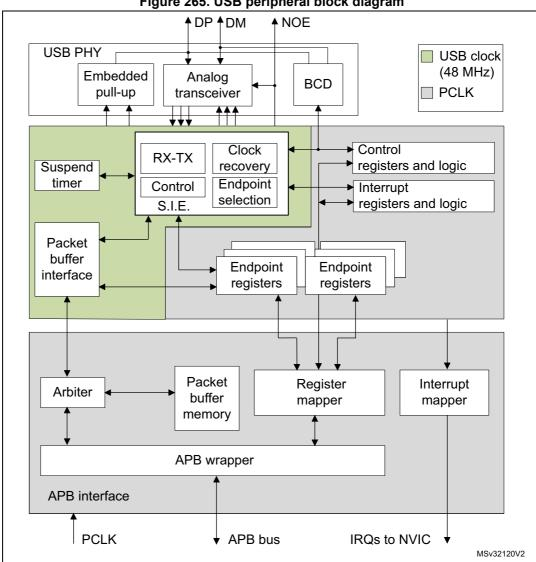
Figure 265. USB peripheral block diagram
