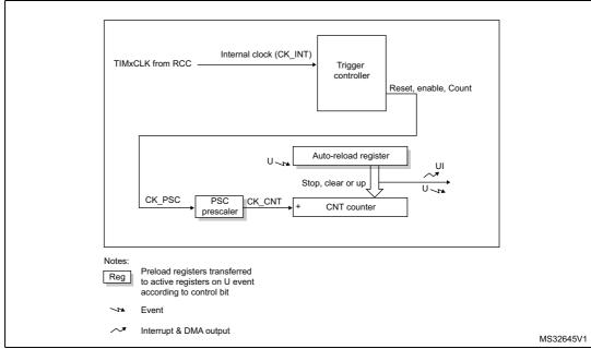
Figure 139. Basic timer block diagram
