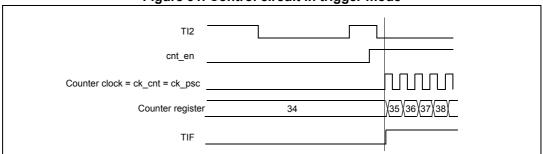
Figure 91. Control circuit in trigger mode
