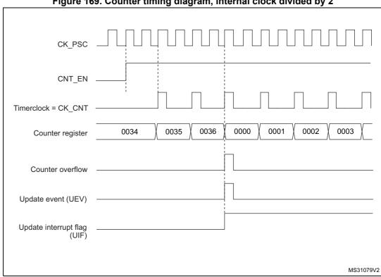
Figure 169. Counter timing diagram, internal clock divided by 2
