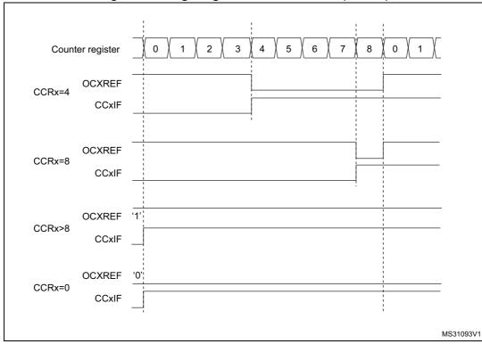
Figure 184. Edge-aligned PWM waveforms (ARR=8)
