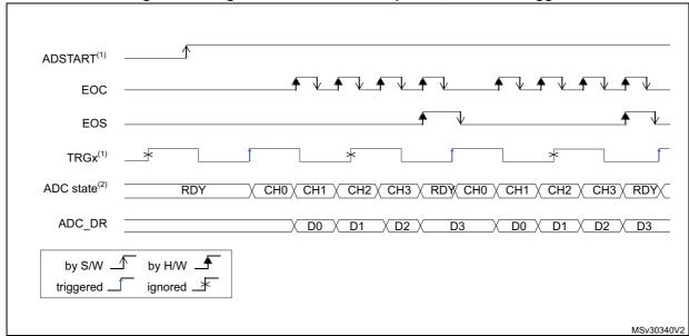
Figure 32. Single conversions of a sequence, hardware trigger
