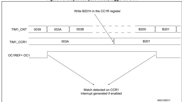
Figure 76. Output compare mode, toggle on OC1
