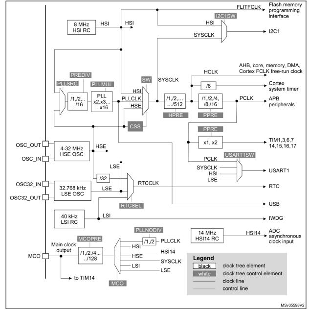
Figure 11. Clock tree (STM32F070x6, STM32F070xB and STM32F030xC)
