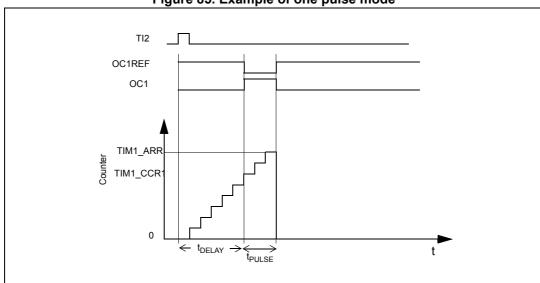
Figure 85. Example of one pulse mode
