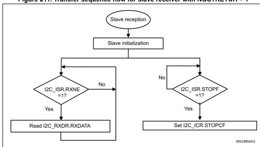
Figure 211. Transfer sequence flow for slave receiver with NOSTRETCH = 1
