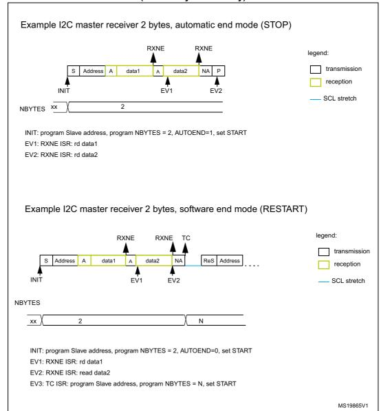
Figure 222. Transfer bus diagrams for I2C master receiver (mandatory events only)
