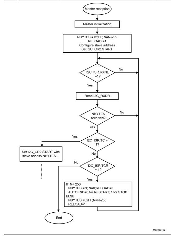
Figure 221. Transfer sequence flow for I2C master receiver for N > 255 bytes
