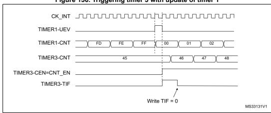
Figure 136. Triggering timer 3 with update of timer 1
