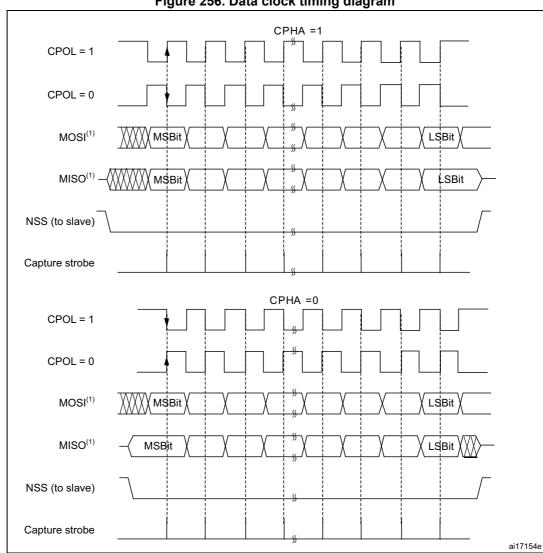
Figure 256. Data clock timing diagram
