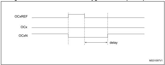
The dead-time delay is the same for each of the channels and is programmable with the DTG bits in the TIMx\_BDTR register. Refer to Section 13.4.18: TIM1 break and dead-time register (TIM1\_BDTR) on page 295 for delay calculation.
