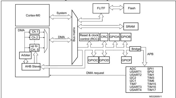
Figure 20. DMA block diagram
