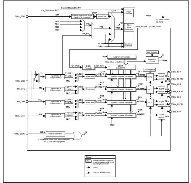
Figure 45. Advanced-control timer block diagram
