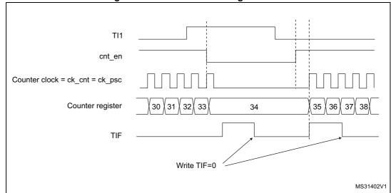
Figure 191. Control circuit in gated mode
