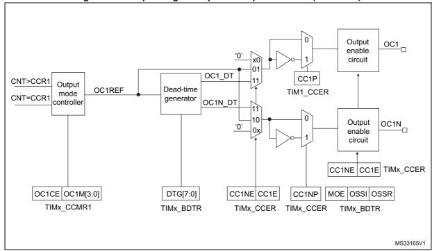
Figure 180. Output stage of capture/compare channel (channel 1)
