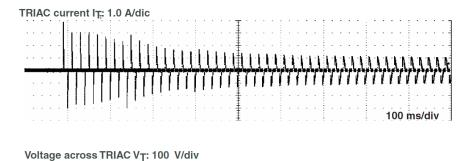
Figure 6. Soft start for 150 W, 230 V incandescent lamp
