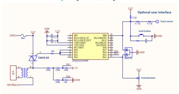
Figure 4. Light dimmer circuit diagram
