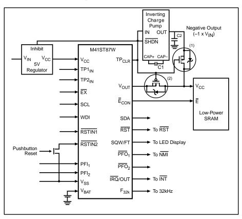
Figure 1: Circuit connections
