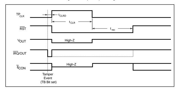
Figure 2: Tamper output timing
