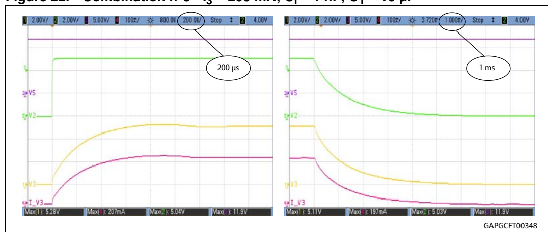
Figure 23. Combination n°5 - C_i = 1 nF; C_1 = 10 \mu F; load switch ON/OFF
