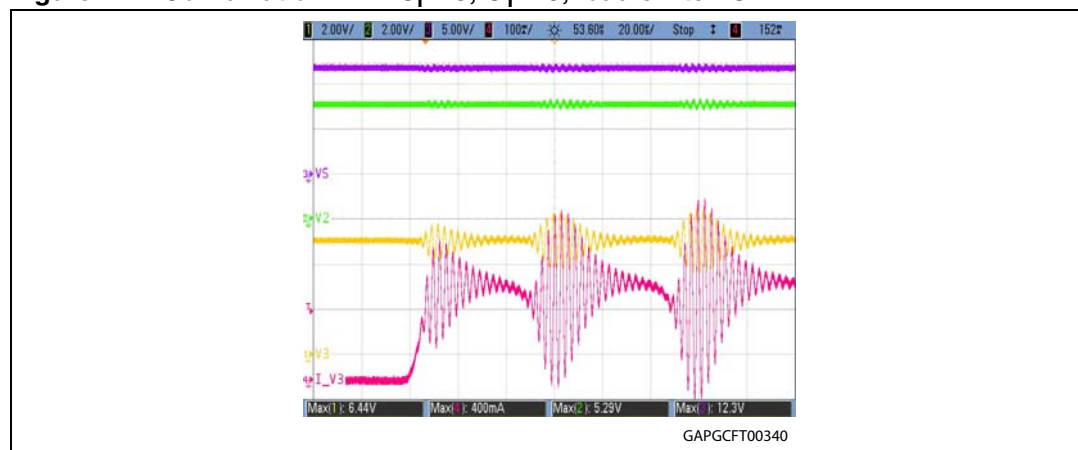
Figure 14. Combination n°1 - C_i = 0 ; C_1 = 0 ; load switch ON
