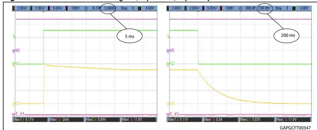
Figure 22. Combination n°5 - I_3 = 200 mA; C_i = 1 nF; C_1 = 10 \mu F
