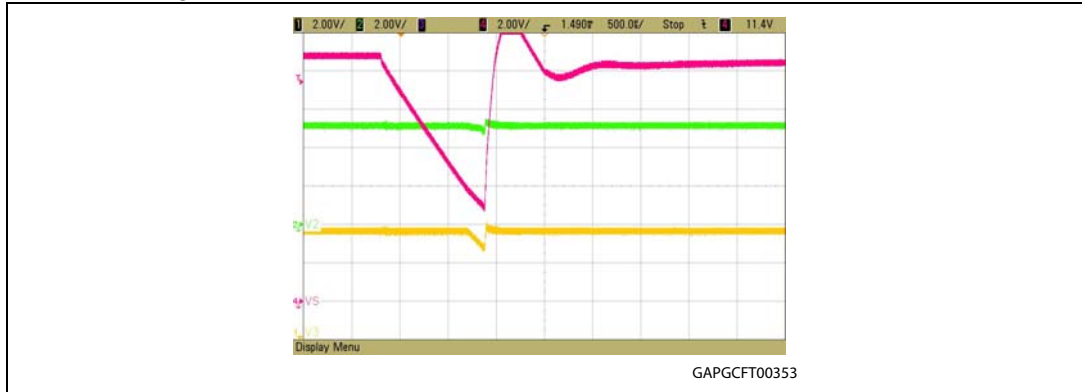
Figure 27. V_S cranking (1 ms pulse)
