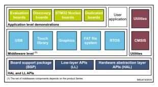
The STM32Cube HAL is an STM32 embedded software layer that ensures maximized portability across the STM32 portfolio, while the LL APIs make up a fast, light-weight, expert-oriented layer which is closer to the hardware than the HAL. HAL and LL APIs can be used simultaneously with a few restrictions.
