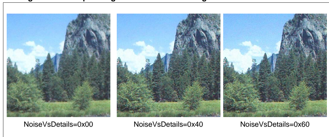
Figure 35. Example images with different settings for noise vs. details slider
