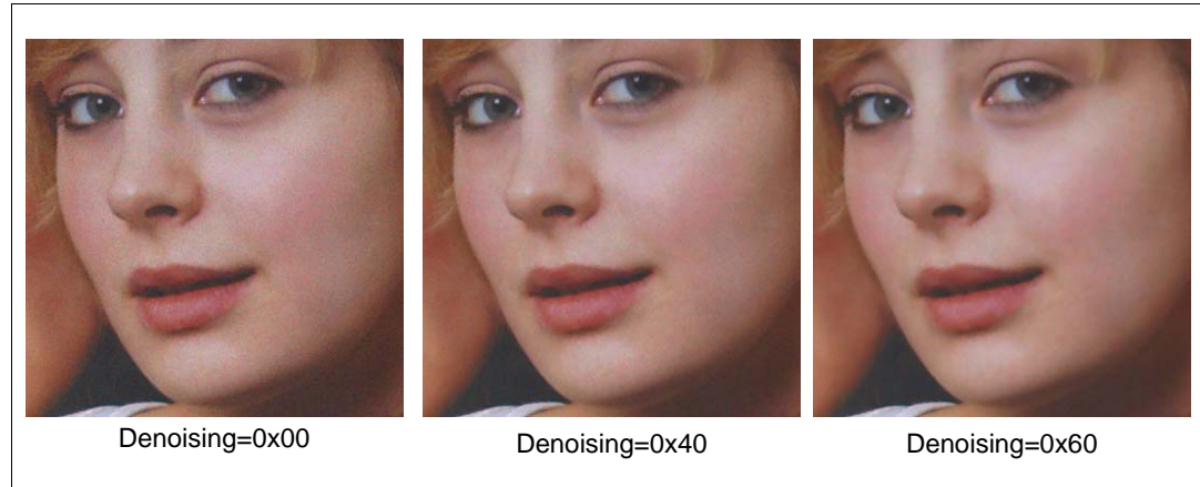
Figure 34. Example images with different settings for denoising slider
