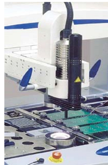
Figure 10. Comintec ONYX32 - Semi-automatic equipment for component rework
