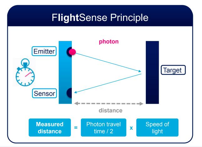
**Fully Integrated Time of Flight Module** True distance measurement Independent of target size, color & reflectance Very fast (few ms) Low power
