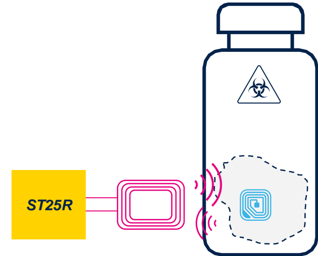
isolated gap communication
