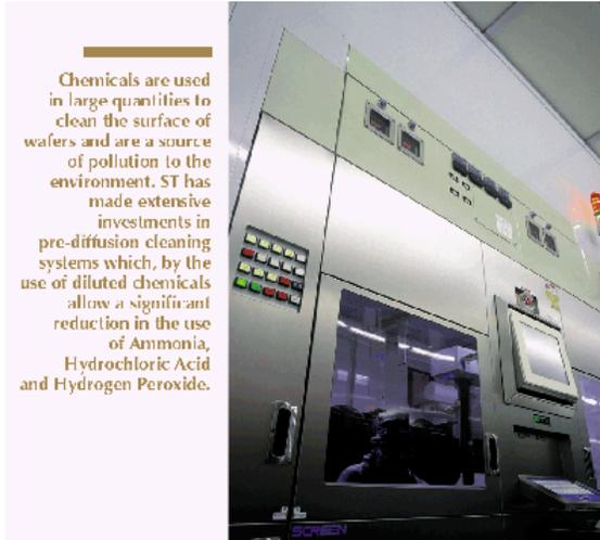
Chemicals are used in large quantities to clean the surface of wafers and are a source of pollution to the environment. ST has made extensive investments in pre-diffusion cleaning systems which, by the use of diluted chemicals allow a significant reduction in the use of Ammonia, Hydrochloric Acid and Hydrogen Peroxide.
