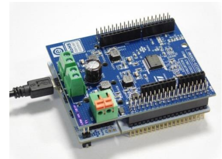
X-NUCLEO-PLC01A1 plugged on a compatible STM32 Nucleo board
