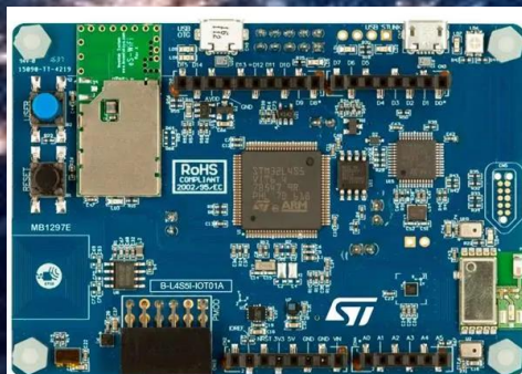
B-L4S5I-HOT01A Discovery kit for IoT Node
