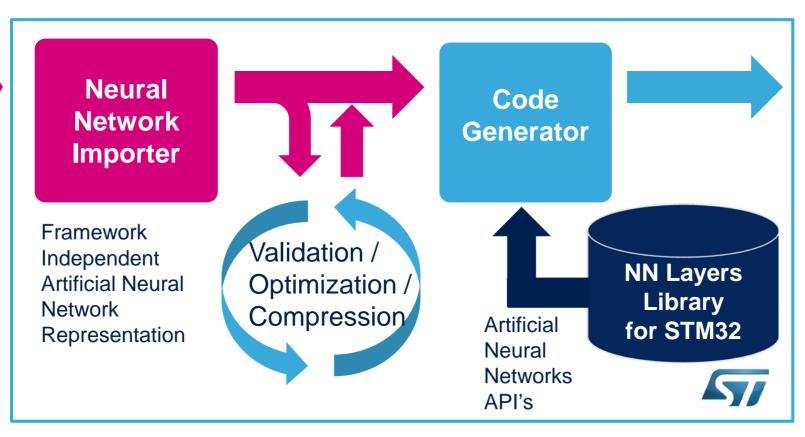
**Embedded Solution Optimized Artificial** Neural Network Code generated for STM32
