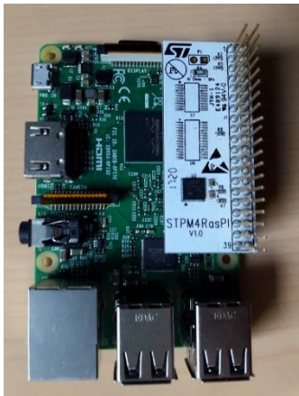
Raspberry Pi® & STM4RasPI expansion board
