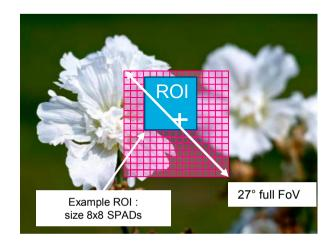
Changing the ROI by software allows to virtually reduce the FoV
