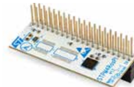
STPM4RasPI TPM expansion board
