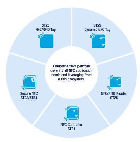
ST's dynamic NFC / RFID tags feature up to 64-Kbit of EEPROM memory which can be accessed either through a low-power I<sup>2</sup>C interface or an RF contactless interface operating at 13.56 MHz. Both short-range (ISO 14443-A) and long-range (ISO 15693) standards are supported:
