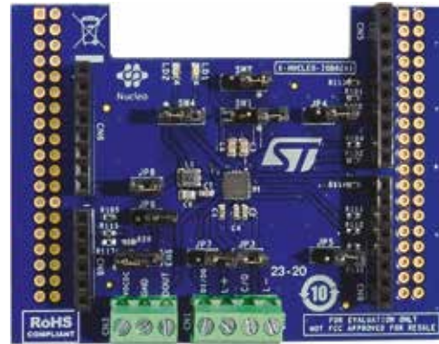
Fig. 9 – X-NUCLEO-IOD02A1 expansion board based on L6364 for STM32 Nucleo
