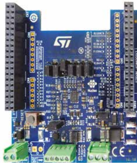
Fig. 5 – The P-NUCLEO-IOM01M1 kit is based on the STEVAL-IOM001V1 (reported in the picture) and the NUCLEO-F446RE
