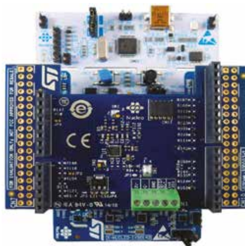
Fig. 7 – The P-NUCLEO-IOD01A1 kit is made of NUCLEO-L073RZ, X-NUCLEO-IKS01A2 and the STEVAL-IOD003V1 (visible on top)
