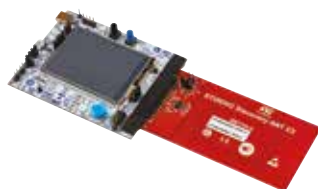
ST25DV64KC-DISCO ST25DV-I2C based NFC tag discovery board
