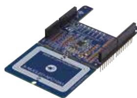
X-NUCLEO-NFC10A1 ST25R200 based NFC reader Nucleo shield board
