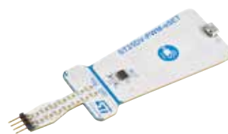
ST25DV-PWM-eSET ST25DV-PWM based NFC tag discovery board
