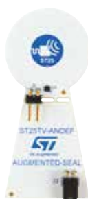
ST25TV02KC-ASEAL ST25TV-based NFC tag evaluation board
