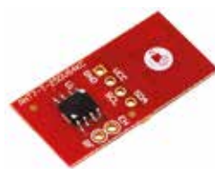
ANT7-T-25DV64KC ST25DV-I2C based NFC tag development board
