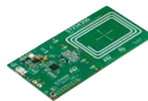
ST25R300-EMVCO ST25R300 based EMVCo 3.x reference design
