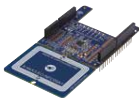
X-NUCLEO-NFC09A1 ST25R100 based NFC reader Nucleo shield board
