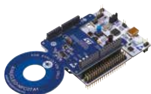
X-NUCLEO-NFC07A1 ST25DV-I2C based NFC tag Nucleo expansion board
