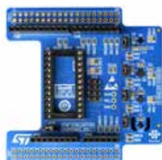
X-NUCLEO-IKS01A1 Motion and environmental sensors
