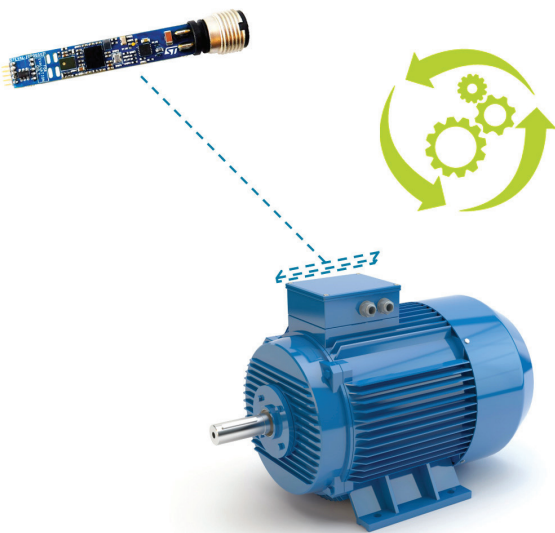
Fig. 11 – Predictive maintenance needs smart sensors, edge processing and industrial protocols
