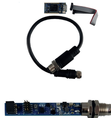
Fig. 9 - STEVAL-IOD04KT1 dual-channel IO-Link reference design kit based on L6364W.
