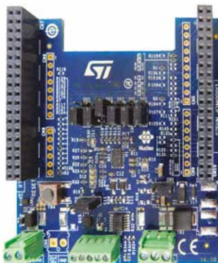
图5 – P-NUCLEO-IOM01M1套件基于STEVAL-IOM001V1（如图所示）和NUCLEO-F446RE
