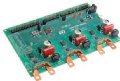
EVALSTPM-3PHISO Three-phase full shunt electricity meter evaluation board based on STPMS2, STISO621 and STM32
