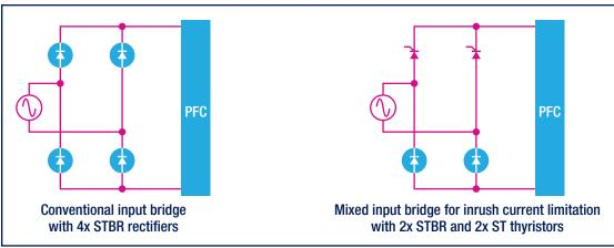
Note: For designs combined with a thyristor, Application Note AN4606 provides additional information about the inrush current limiter function on st.com
