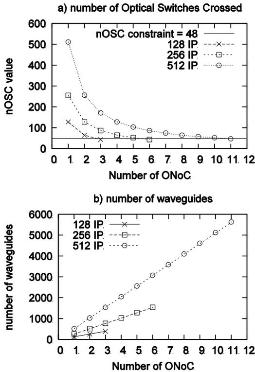
Figure 5 Scalability of the method: a) nOSC and b) number of waveguides
