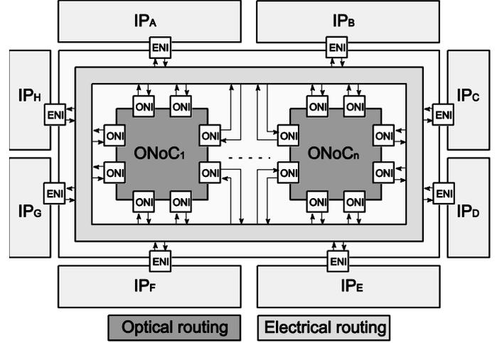
Figure 2 Multi-ONoC architecture interconnecting 8 IPs through  $n$  ONoCs.
