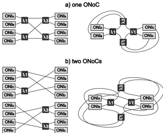
Figure 4 Schematic view and layout for a) one ONoC and b) two ONoCs scenarios
