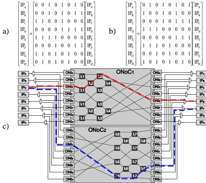
Figure 3 a) ONoC<sub>1</sub> and b) ONoC<sub>2</sub> connectivity matrixes and c) the resulting Multi-ONoC architecture
