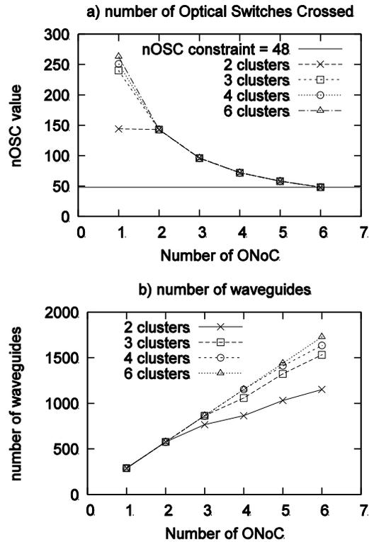
Figure 6 Efficiency of the method for interconnecting 288 clustered IPs: a) nOSC and b) number of waveguides
