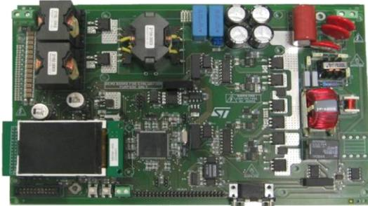
Figure 8: STEVAL-ISV003V1, 250 W microinverter for plug-in PV panels
