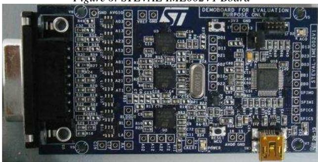
This family of boards is composed of two evaluation boards: the STEVAL-IME002V1 and the STEVAL-IME002V2 respectively designed to demonstrate the use of HM301D in Electrocardiographs (or patient monitor systems) (ECG) and Automated External Defibrillator (AED) configurations. They also host a 32-bit microcontroller of the STM32 family that manages the SPI protocol of HM301D and the USB communication from/to the PC. Any board could be easily used with dedicated PC
