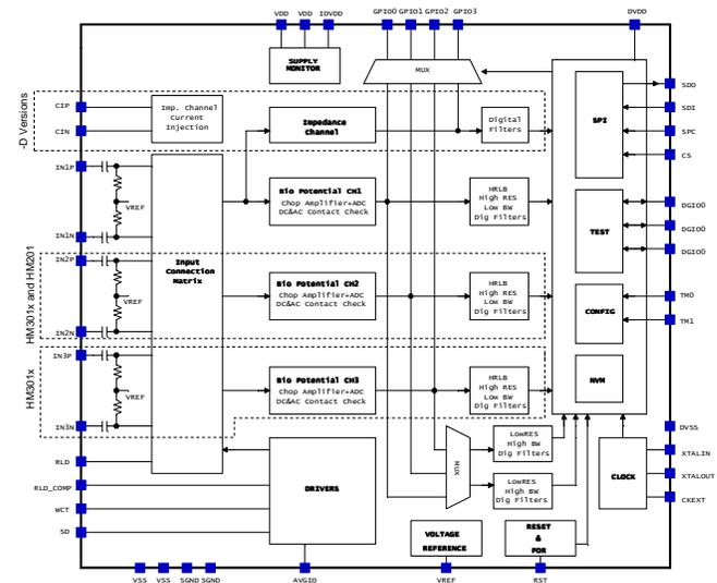
The ST HM301D (see Figure 4) provides a suitable solution for the ECG signal acquisition by offering, in addition to the above mandatory features, a series of fully integrated and configurable digital band-pass filters that allow selective analysis of the ECG wave by physicians.
