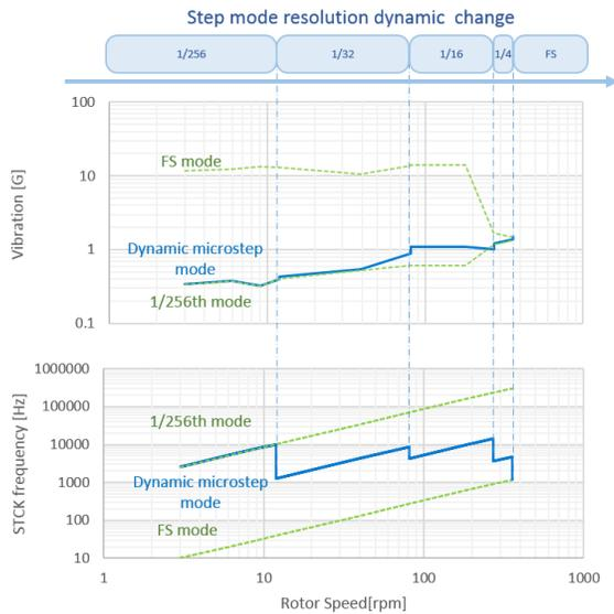
Figure 6: Scaling step clock and microstepping resolution
