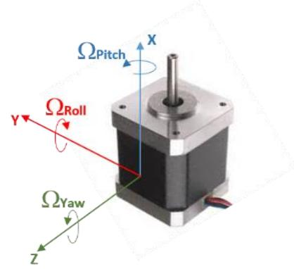
Figure 2: Axes orientation of the inertial module on the motor
