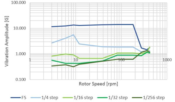
Figure 5: Vibration VS speed at different microstepping resolution
