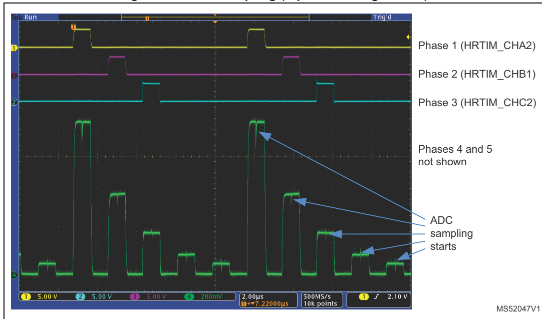
Figure 24. ADC sampling (5-phase configuration)
