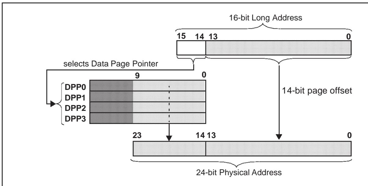
Figure 2 Interpretation of a 16-bit long address
