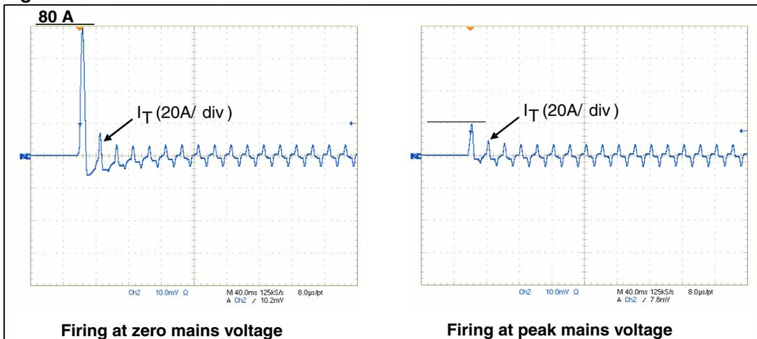
Triac turn on at peak mains voltage allows the reduction of the peak inrush current by 75% compared to a zero voltage switch on as shown in [Figure 8](#).
