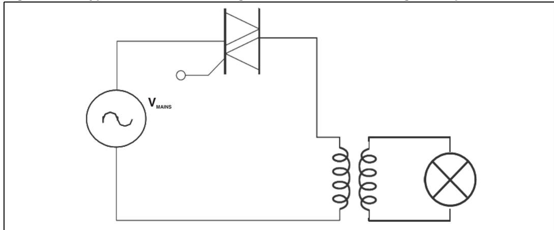
Like microwave oven transformers, transformers for lighting application present an overcurrent if they are switched on at zero voltage due to magnetizing current.
