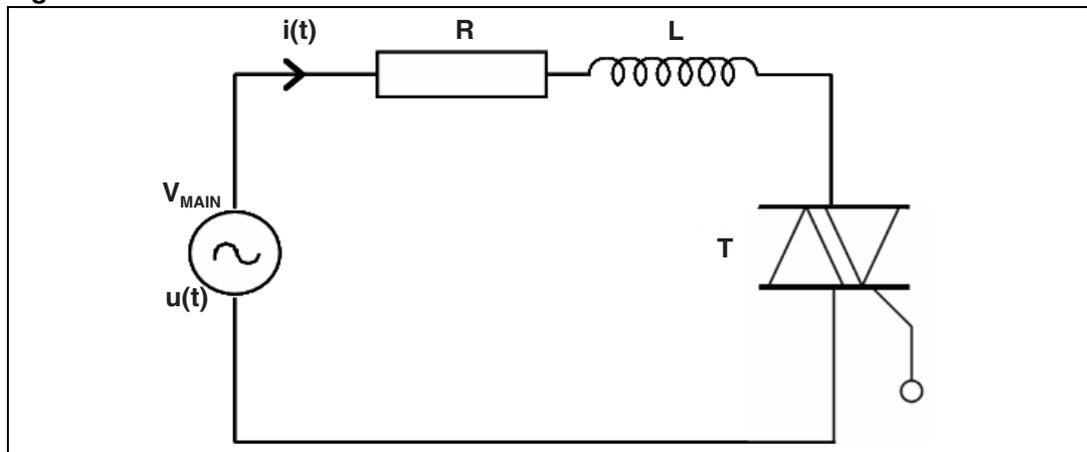
According to [Figure 1](#), the AC load current  $i(t)$  is define by [Equation 1](#).
