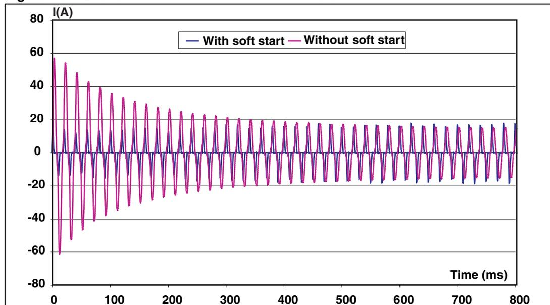
Figure 10 show an example of Triac switching on a 2200 W universal motor with or without soft start. The difference is very clear, the current reaches a peak current up to 60 A without soft start while it reaches 10 A with soft start. This current reduction has a direct impact in the AC switch maximum junction temperature as shown in Figure 11 with a T1050H Triac.
