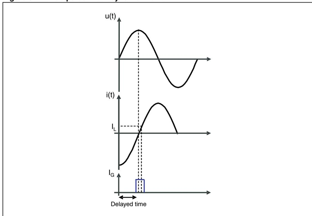
In case the zero line voltage event is not sensed by the Triac control circuit or no timer is available to manage triggering times, one solution is to apply a DC gate current. In this case the average current consumption for the power supply will be higher. But today more and more switching mode power supplies (SMPS) are used offering a higher output current capability.
