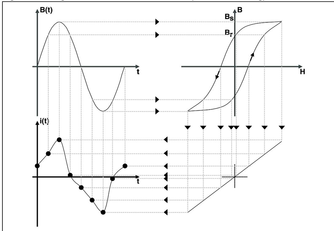
According to [Equation 2](#), at start up at zero voltage the current is higher (longer time to integrate voltage and so higher induction reached in the 1st cycle) and so there is a higher risk of reaching magnetic core saturation.
