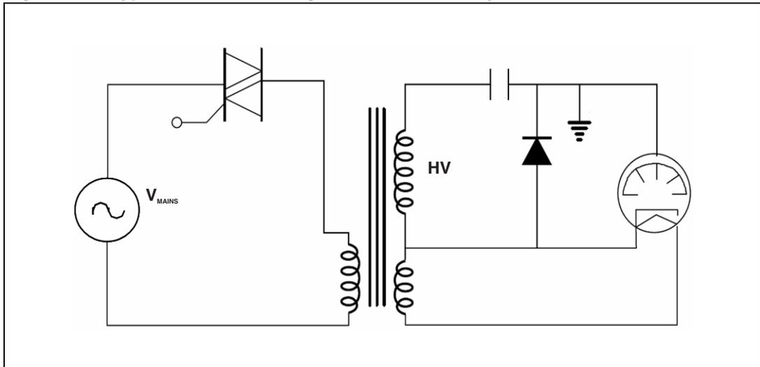
The power to be controlled is typically between 1 to 2 KW and the nominal rms current is in the range of 10 to 20 A according to the line voltage. The inrush current comes from the magnetizing current through the transformer at turn on.
