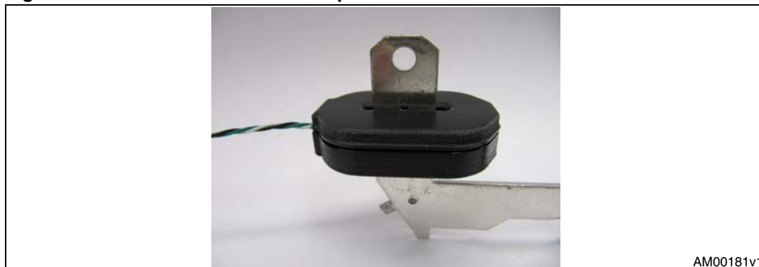
Figure 4. Pulse current sensor adapted for a flat buss bar
