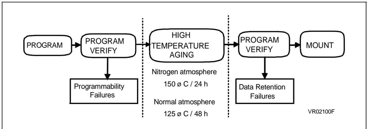
Screening devices that are subject to data retention failures will allow customers to obtain OTP devices with a similar quality level compared to ROM devices.
