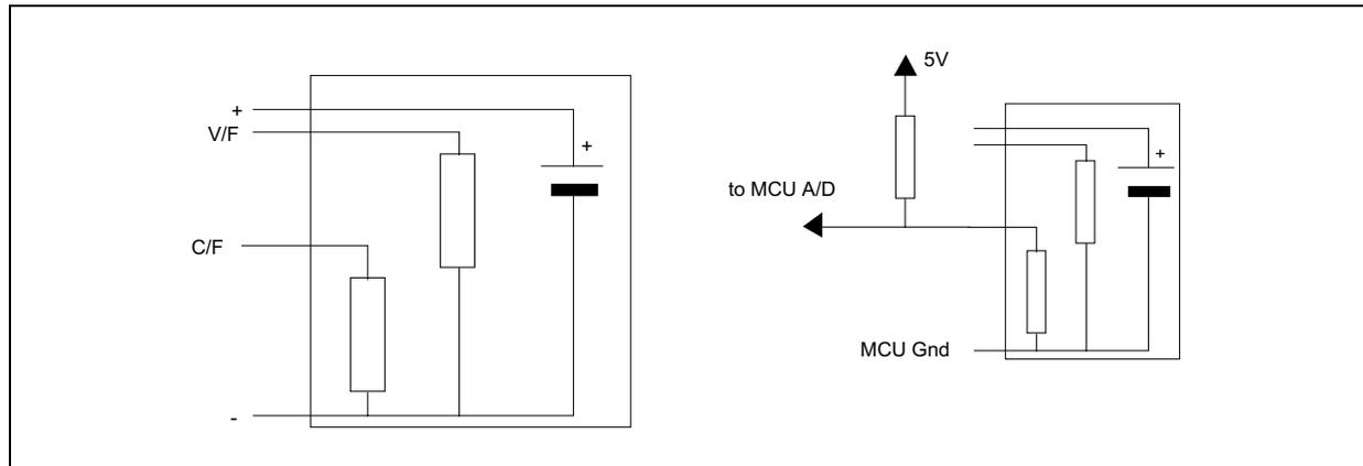
Table 1 : BATTERY VOLTAGE DETECTION FROM V/F
