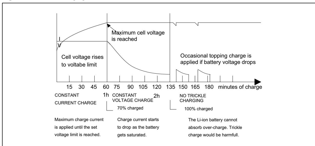
During Stage 1, the battery is charged at constant current. The battery voltage is slowly increasing from original voltage up to the maximum cell voltage, which depends on the battery electrode technology (4.2V/cell for coke electrode, 4.1V/cell for graphite electrode).
