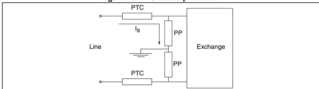
The PTC thermistor is a device which operates through a very rapid resistance increase as a function of the temperature.
