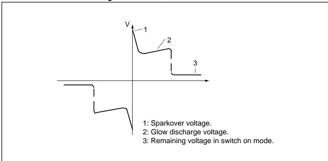
The major disadvantage of this kind of device is its response time, in fact the maximum voltage across the gas tube depends on the  $dv/dt$  of the surge.
