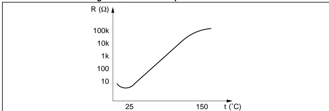
The major disadvantage of the fuse does not exist with the PTC device. Unfortunately this kind of component has a large tolerance, a long time to return to its stand off point and a drift of its value.
