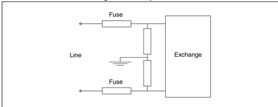
The fuse is a classical case of protection by opening the circuit. [Figure 11](#) shows an exchange protected by fuses and [Figure 12](#) represents an example of the limit curve of the fusing action.
