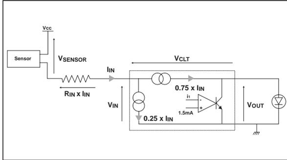
To calculate the drop voltage across the CLT device, the circuit of *figure 3* gives the following equations:
