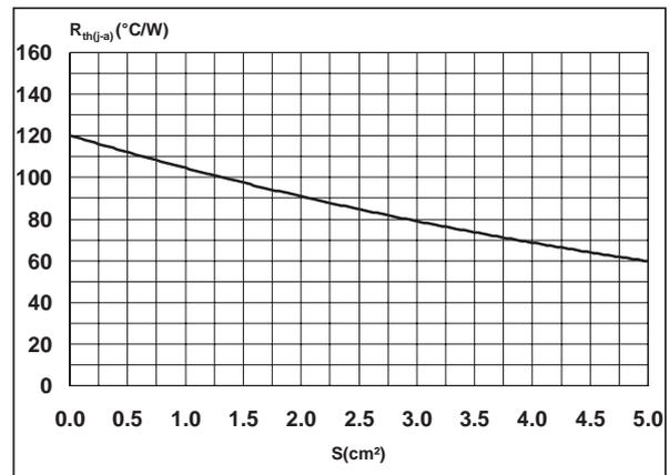
As an example, the copper surface on the demo board is equal to  $1.2cm^2$  allowing operation ambient temperature up to  $100^{\circ}C$ .
