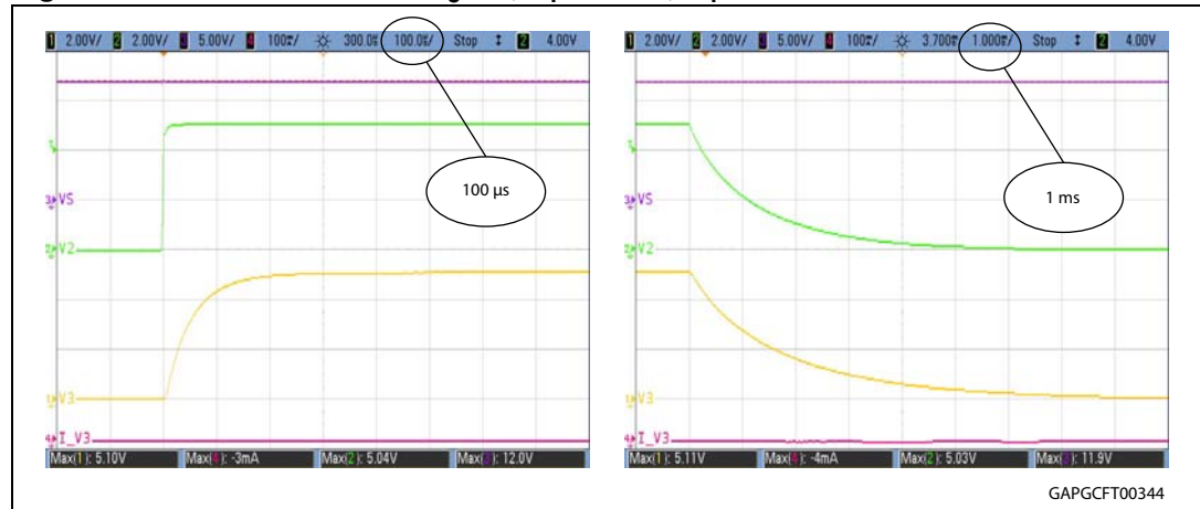
Figure 19. Combination n°3 - I_3 = 200 mA; C_i = 10 nF; C_1 = 0
